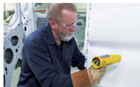
Video Three - Transit Side Panel Repair
